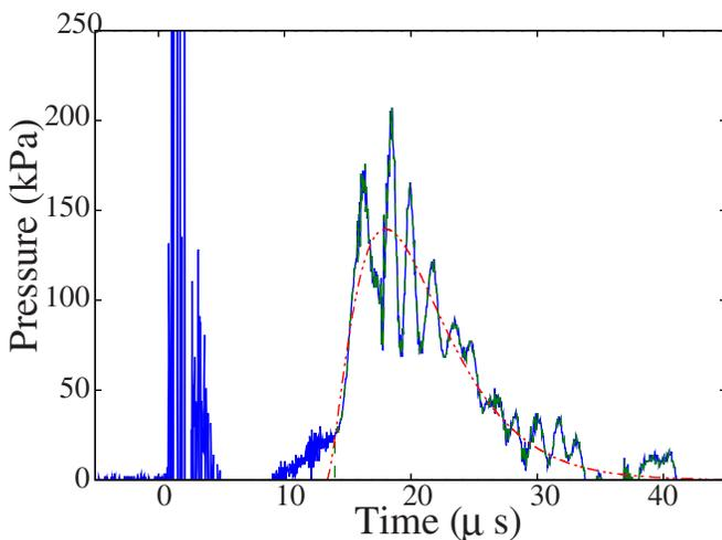
FIG. 2. (Color online) Sample pressure probe trace. We trim the raw signal (solid line) to remove the initial noise. The resulting curve (dashed, rising from zero near 13  $\mu\text{s}$ ) is fitted to Eq. (1) (dot-dot-dashed, smooth curve). Traces are compared based on the fitted curves.
