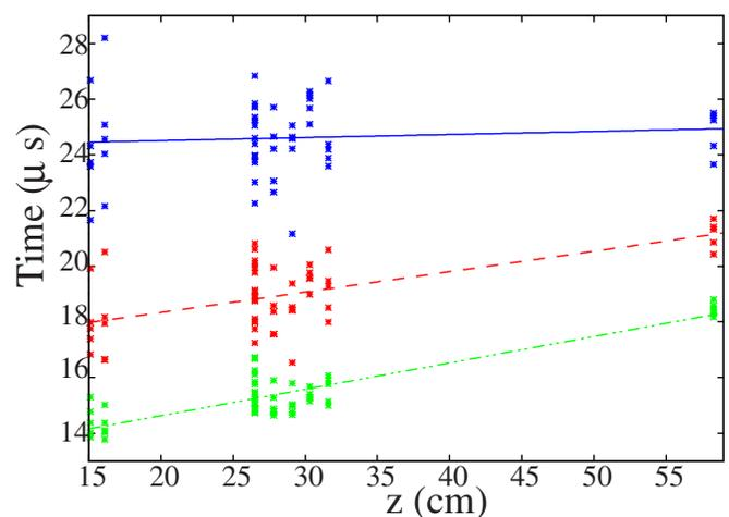
FIG. 4. (Color online) Pressure wave timing as a function of position. The lowest data set is arrival time  $t_{\text{rise}}$ . The middle data set shows the time  $t_{\text{pk}}$  of peak pressure. The top data set shows the time  $t_{\text{fall}}$  of the pressure decrease. Points show individual measurements. The lines are linear fits.
